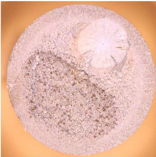
Fracture surface of axial composite sample
