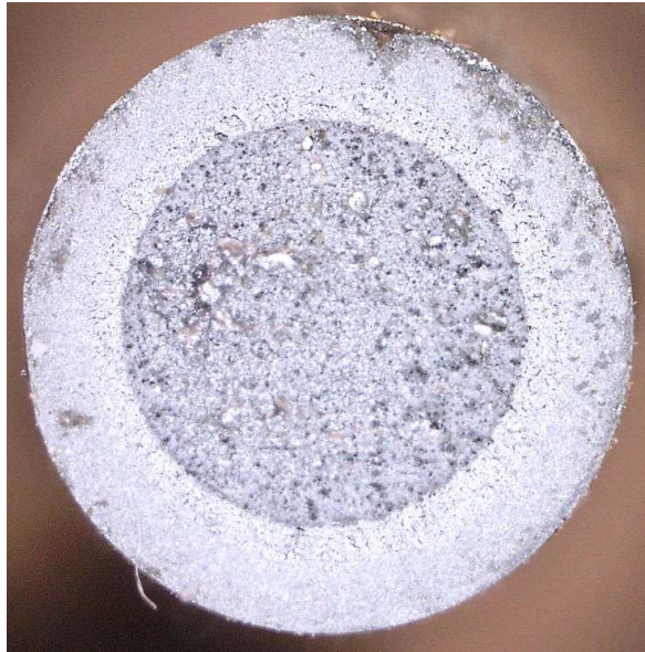
Axial sample with surface failure
