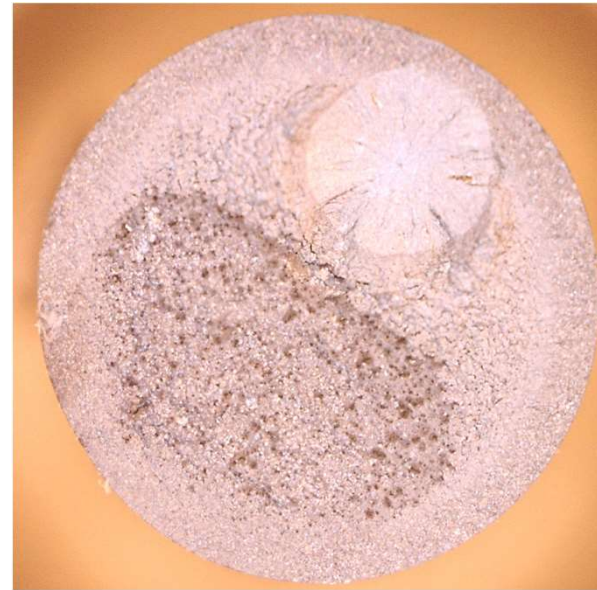
Axial sample with fisheye failure
